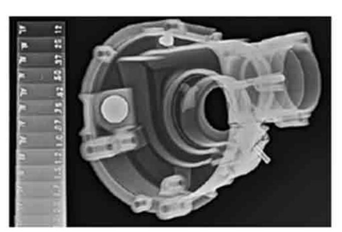
The steel housing is ideal for the industrial environment of NDT applications. All standard film formats can be digitized, up to a width of 35 cm (14 in.), without length limitation in resolutions between 50  $\mu$ m and 500  $\mu$ m. The FS50B is the first and only digitizer on the market that handles the full density range in one working range with the requested contrast sensitivity.
