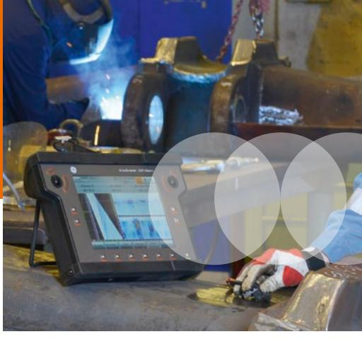
the USM Vision+ even comes with an integrated stylus to support inspections where gloves are required. Its robust, rubberised housing is sealed to an IP 54 rating, to resist dust and humidity. It has a hot swap battery to keep your inspection going despite battery changes. And at just 4,5 kg (9.9 lbs) including batteries, the USM Vision+ is truly portable.
