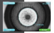
With the first click the software will identify the circle that best fits on the indentation edge, draws it over the indentation image, records its diameter and calculates the Brinell number
