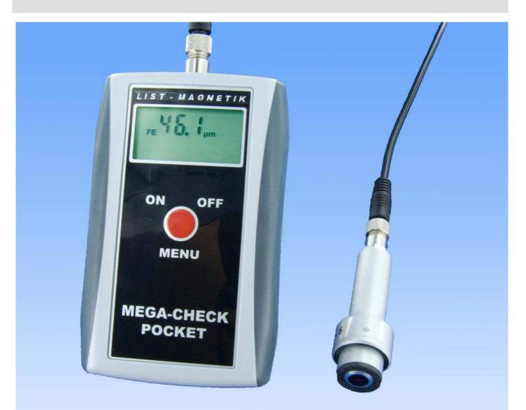
The new **MEGA-CHECK** *Pocket* devices use digital measuring probes, in which the analog signals are digitised directly in the probe and transferred digitally via the probe cable to the measuring device. This new technology is very immune to interference and makes high accuracy, reproducible measurements possible.
